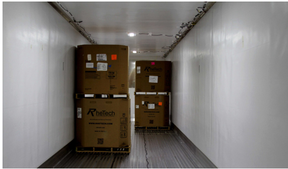
This image shows how the traditional arrangement of recessed ceiling dome lights in a 53' trailer cause many dark areas from cargo shadows.
