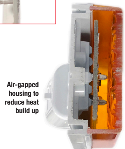
Pin connections are insert molded into the housing eliminating moisture intrusion
